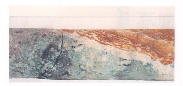
PLATE 4. Redox front at 42.0 m; drillcore F1. Nodular pitchblende on reduced side of front (black circle), kaolinite-rich layer (white layer) separating reduced (grey) and oxidised (brown) rock.
