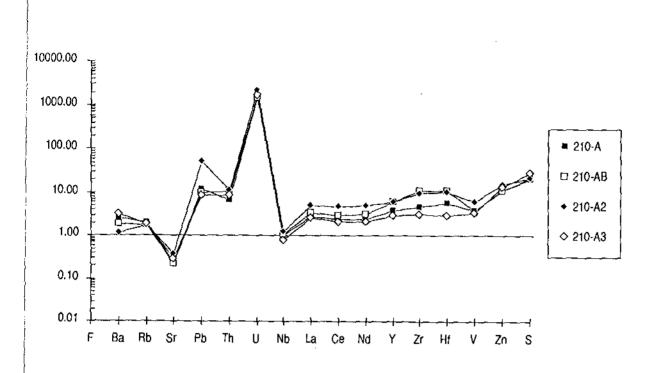
Figure 33. Trace element compositions of the highly mineralised breccias at 210 m from borehole F4 normalised to the average composition of unaltered regional samples.
