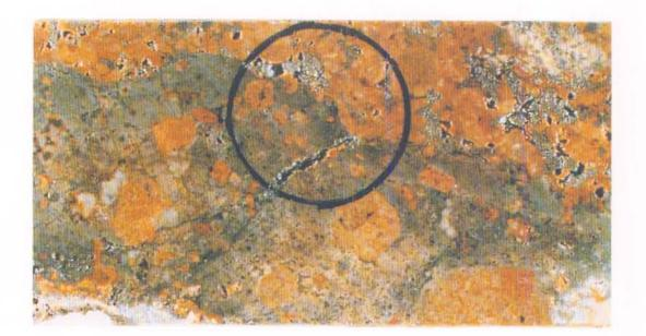
PLATE 1:1-6. Post-breccia fractures (circle) and pores from a nepheline syenite fragment in reduced breccia mineralised with fresh-yellow and silver-grey (galena-like material) coated pyrites (sample 6; F4/382.49 – 382.63 m; 383-1A; scale: circle  $\emptyset = 27$  mm).
