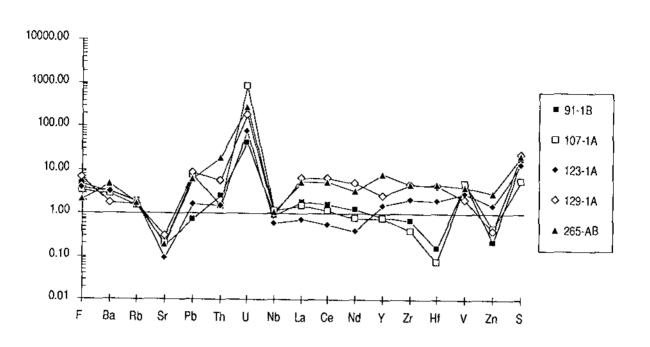
Figure 25. Average trace element compositions of hydrothermally altered, reduced nepheline syenite xenoliths from borehole F4 normalised to the average composition of unaltered regional rocks.
