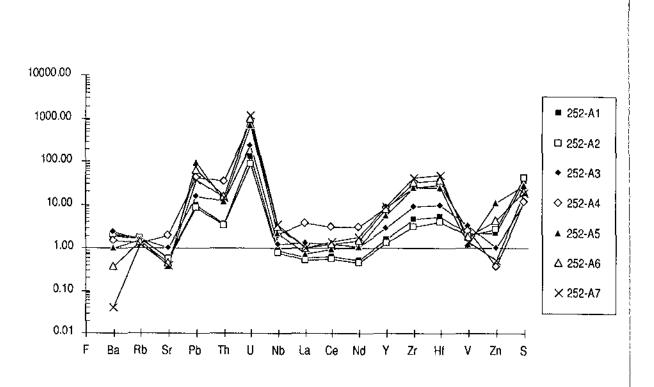
Figure 35. Trace element compositions of the highly mineralised breccias at 252 m from borehole F4 normalised to the average composition of unaltered regional samples.
