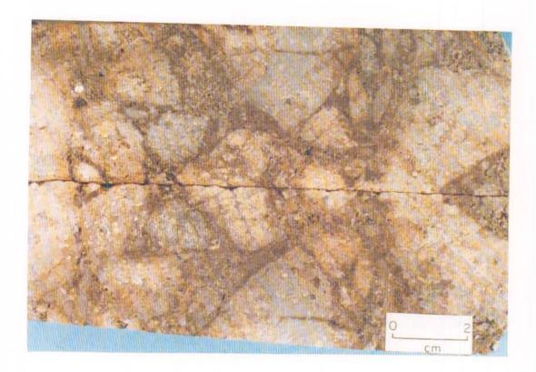
PLATE 1:1-11. Reduced, strongly pyritised breccia matrix in clast-supported breccia. Note microporosity of breccia matrix. The syn-breccia matrix pyrites are fine-grained and around 0.2 mm in size (sample 11; F4/414.10 – 414.24 m).
