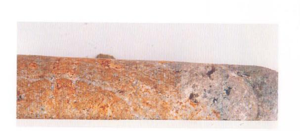
PLATE 3. Redox front at 33.5 m; drillcore F1.
