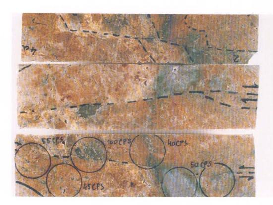
PLATE 1:1-4. Reduced breccia with hydrothermal Zr (-REE)-U-pyrite (-sulphides) mineralisation (black-coloured circles) disrupted by post-breccia fracturing. Pyrites are microcrystalline and aggregated with other ore minerals. Incipient recent light-grey sulphate and bluish secondary Mo-mineral/ilsemannite alteration products [e.g. enclosed by 50 cps-circles (sample 4; F4/242.57 – 242.95 m; 243-1A; scale: circle  $\emptyset = 27$  mm)] are also present.
