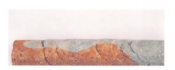
PLATE 5. Redox front at 66.1 m; drillcore F1.
