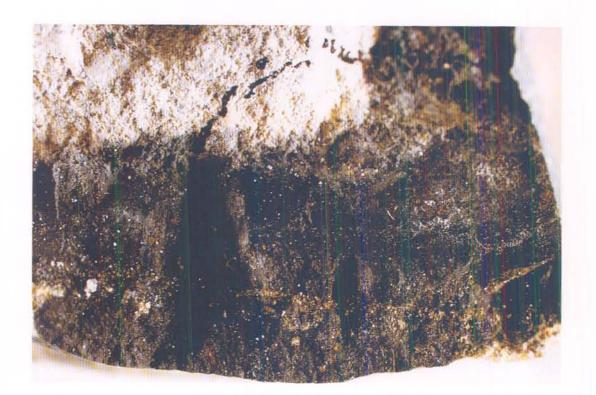
PLATE 1:1-16. Detail of massive pitchblende nodule VII (Plate 1:1-15) showing syn-pitchblende pyrites within the massive pitchblende zone (sample 18; VII; about 3.4 x nat. size).
