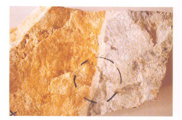
PLATE 1:1-12. Hand specimen of U-mineralised redox front in fine-grained phonolite. Note white versus light-grey (with darker nodules) coloured front of total pitchblende dissolution and white versus yellow-brown front of HFO (hydrous ferric oxides, mainly limonite) precipitation. Pyrites were selectively extracted from the fine-grained reduced phonolite avoiding the pitchblende nodules (sample 13; about 1.6 x nat. size).
