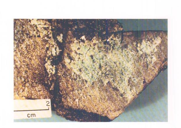
PLATE 1:1-18. Recent sulphates (bluish-whitish needles and dense mass) from a strongly pyritised phonolite (sample 20; M-1).
