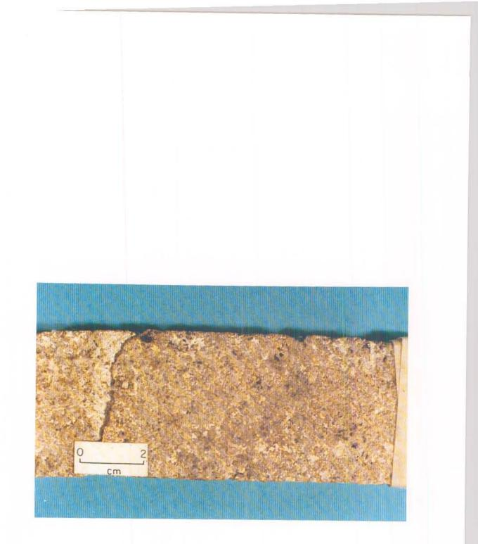
PLATE 1:1-1. Reduced medium- to coarse-grained hypabyssal phonolite from a conductive zone. Note open porosities and white clays. The rock is rich in pyrite. Pyrites are of max. grain-size ~0.5 mm and occur disseminated throughout the rocks and in the pores (sample 1; F1/69.43 – 69.63 m).
