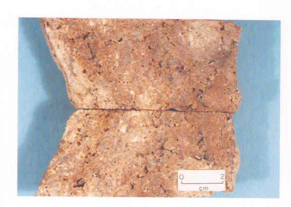
PLATE 1:1-10. Reduced, strongly porous and pyritised medium-grained phonolite xenolith (of breccia). Pyrite grain-sizes are around 1.0 mm (sample 10; F4/407.57 – 407.67 m).
