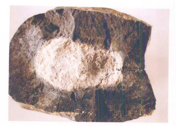
PLATE 1:1-15. Massive pitchblende nodule with silicate core (white) and massive pitchblende zone containing disseminated medium-grained pyrites (sizes Ø: 0.5 – 1.5 mm) of syn-pitchblende origin. Lower right-hand corner of nodule is shown in more detail in Plate 1:1-16 (sample 18; VII; about 1.7 x nat. size).
