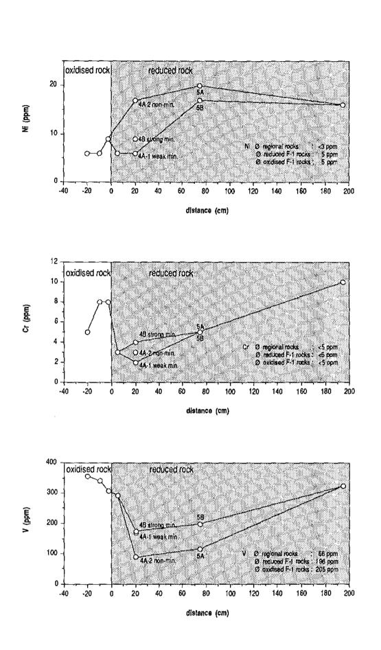
Figure 6-12. RFI redox front: geochemical distribution of Ni, Cr and V.
