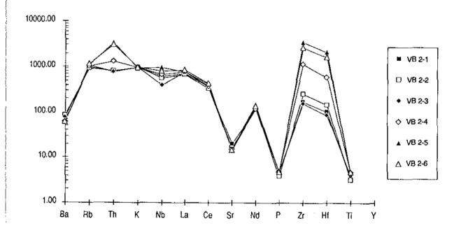
Figure 40. Incompatible elements normalised to chondrite and primitive mantle of the mineralised breccias in contact with the nepheline syenite xenolith at 353 m from borehole F4 (normalisation factors from Thompson, 1982).
