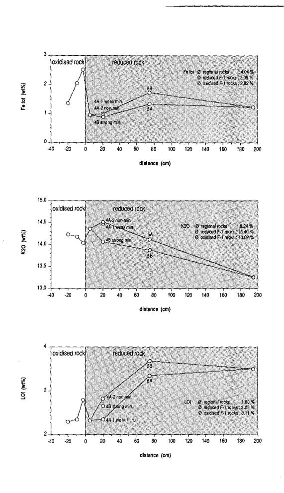
Figure 6-4. RFI redox front: geochemical distribution of Fe<sub>2</sub>O<sub>3(101)</sub>, K<sub>2</sub>O and LOI.
