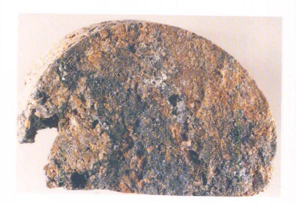
PLATE 1:1-7. Post-breccia fracture (in reduced breccia) mineralised with silvery-grey coated and uncoated pyrites and minor white clays (sample 7; F4/385.40 – 385.64 m; 386-1A; 2.5 x nat. size).
