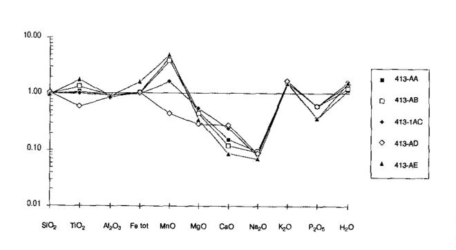
Figure 19. Average major element composition of hydrothermally altered, reduced nepheline syenite xenolith at 413 m depth from borehole F4, normalised to the average composition of unaltered regional rocks.
