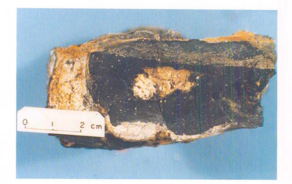
PLATE 1:1-14. Massive pitchblende nodule showing the silicate core (whitish) surrounded by the main pitchblende zone (black) and a discontinuous external silicate shell (whitish). The pitchblende zone contains, in the upper part of the photograph, a layer of pyrite (yellowish) of post-hydrothermal and pre-pitchblende origin. Coarse pyrites of syn- pitchblende origin (sample 15; S/N-24) are disseminated throughout the pitchblende zone.
