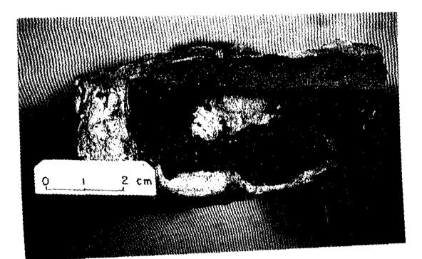
PLATE 3:9-8. Sawn surface of the nodule illustrated in Plate 3:9-7. The nodule consists of a white coloured core of hydrothermally altered and argillised rock (phonolite), surrounded by a black nodule-forming pitchblende zone and a fine external yellowish white clay shell. Note the "horizontal" zone which is extremely rich in secondary coarse-grained pyrites in the top portion of the pitchblende zone (yellow reflectivity). This probably represents a former water table-related phenomenon.
