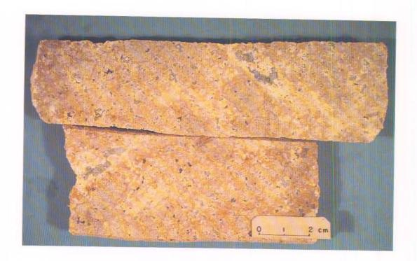
PLATE 1:1-3. Reduced subvolcanic phonolite with minor nepheline syenite pegmatoids of minor microporosity. Pyrites of mean grain-size ~0.25 mm are finely disseminated throughout the rock and in the pores. The analysed pyrite concentrate was separated by N. Waber (Univ. Bern) and identified as "matrix pyrite" (sample 3; F1/125.30 – 125.41 m).
