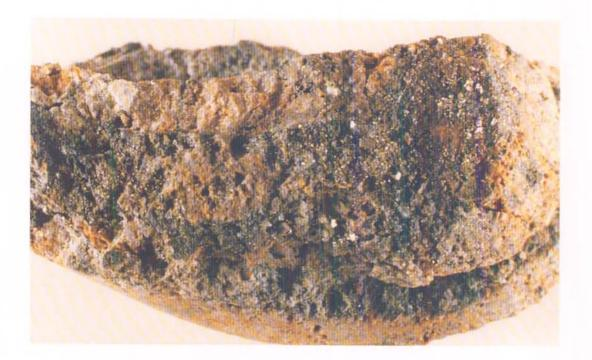
PLATE 1:1-8. Post-breccia fracture (in reduced nepheline syenite xenolith) mineralised with silvery-grey coated and uncoated pyrites (sample 8; F4/394.42 – 394.60 m; 394-1A (?); 2.5 x nat. size).
