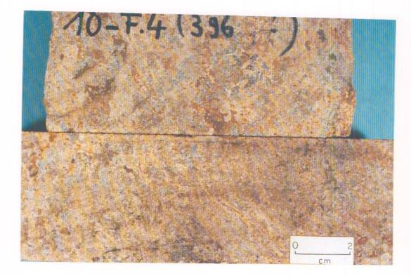
PLATE 1:1-9. Reduced transitional phonolite to nepheline syenite xenolith of breccia, very weakly microporous and non-fractured with finely disseminated pyritisation (max. dimensions of pyrites  $\leq 0.3$  mm) and argillised (sample 9; F4/396.57 – 396.83 m).
