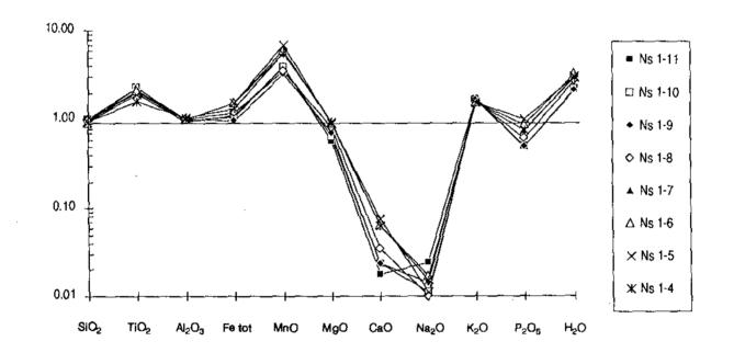
Figure 18. Average major element composition of a hydrothermally altered, reduced nepheline syenite xenolith at 353 m depth from borehole F4, normalised to the average composition of unaltered regional rocks.
