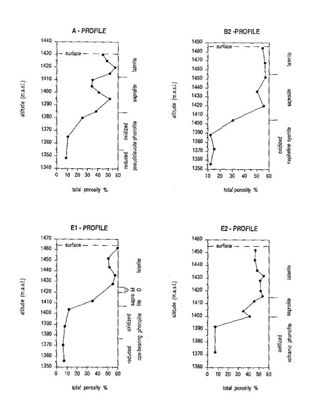
Figure 8. Variation of total porosity in four weathering profiles from different parent rocks. (Profile locations are indicted in Figure 4).
