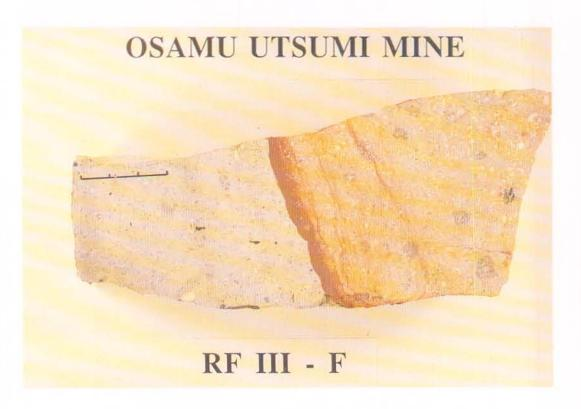
PLATE 8. Redox front RFIII; mine exposure. Mineralised front in dense leucocratic phonolite; small black nodules are located along fissures on the reduced side of the front (scale in cm).
