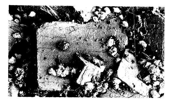
Figure 52. Scanning electron micrograph (SEM 2814/4) of idiomorphic monazites on pyrite. (Reduced leucocratic phonolite at 111 m from borehole F1).
