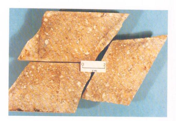
PLATE 1:1-2. Reduced porphyritic phonolite. Pyrites of mean grain-size ~0.25 mm occur finely disseminated throughout the rock and in the subordinate micropores (sample 2; F1/113.65 – 113.79 m).
