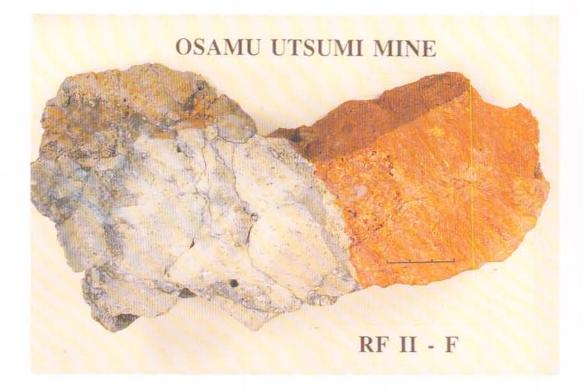
PLATE 7. Redox front RFII; mine exposure. Non-mineralised front in volcanic breccia (scale in cm).
