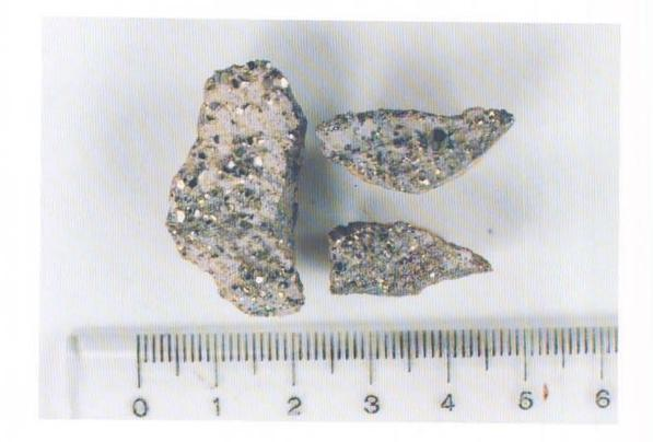
PLATE 1:1-5. Pyritised and argillised (white kaolinite clays) post-breccia fracture in reduced breccia (sample 5; F4/276.15 m).
