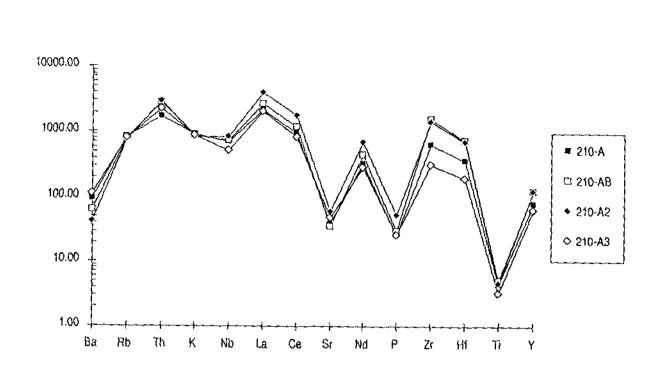
Figure 37. Incompatible elements normalised to chondrite and primitive mantle of the highly mineralised breccias at 210 m from borehole F4 (normalisation factors from Thompson, 1982).
