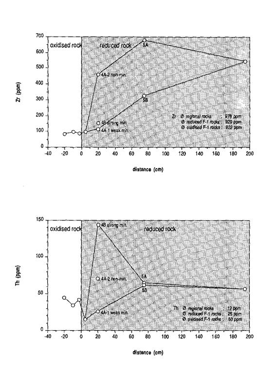
Figure 6-8. RFI redox front: geochemical distribution of Zr and Th.
