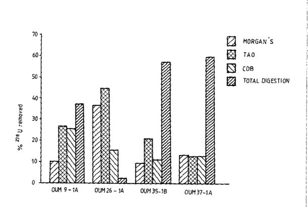
Figure 2-1. The percentage of total U removed by a particular extractant representing a particular phase(s), i.e. minus the uranium removed by the previous extractant.
