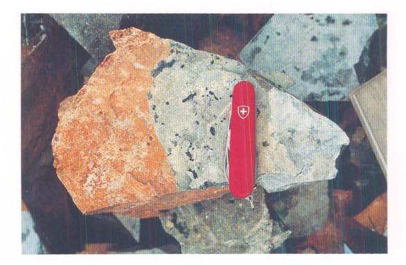
PLATE 6. Redox front RFI; mine exposure. Highly mineralised with black pitchblende nodules on reduced side of front; circular white areas in the oxidised rock (yellow-brown) represent relicts of dissolved pitchblende nodules.
